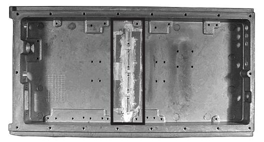
Figure 2 Correct Placement Of Heatspreader On Heatsink
