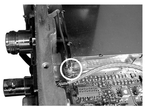
Figure 1 Junction Of Fan Power Feed Wire And Fan Modification
