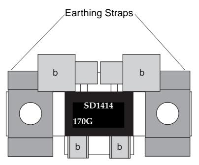
Figure 4 T889 Capacitor/Transistor Placement
